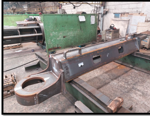
Figure 14. Result of full welding idler and motor bracket body frame
