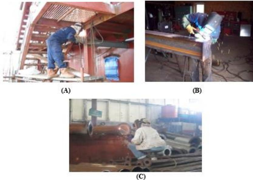
**Gambar 9.** (A) Proses Pengelasan Tipe Vertical (B) Proses Pengelasan Tipe Down Hand (C) Proses Pengelasan Tipe Upper Hand
