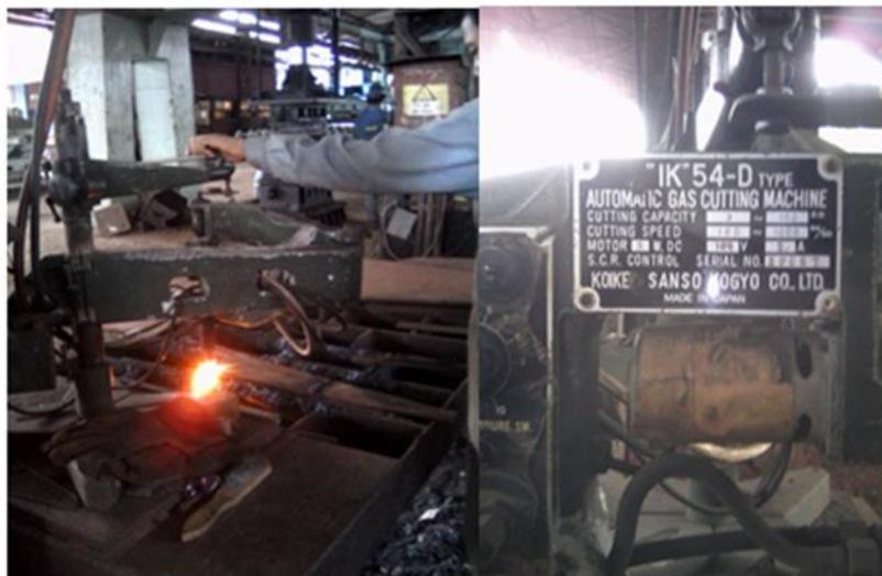
**Gambar 5.** Proses Cutting (Automatic Gas Cutting Machine)
