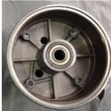
**Gambar 1.** Tromol rem sepeda motor
