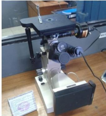
**Gambar 3.** Alat Uji *Metallurgical Microscope*
